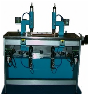
SPINTRONIC stacker: drilling, pin insertion. PAKTRONIK stacker without drilling.
