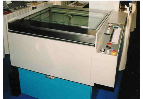
SACK UV-exposure 5 kW, surface 92 x 72 cm
